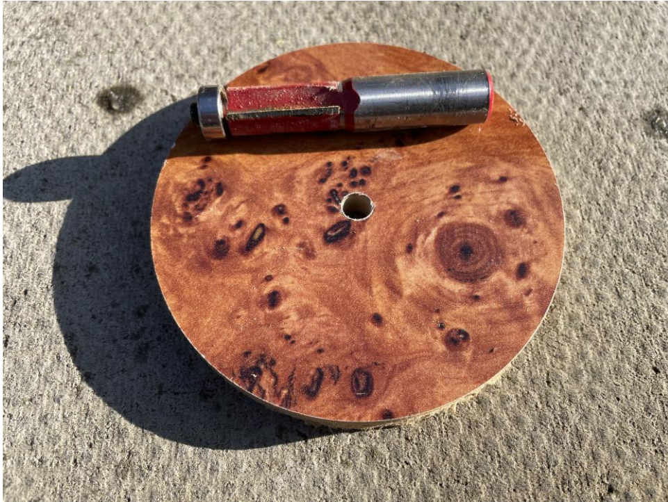
A bearing guided parallel cutter.
