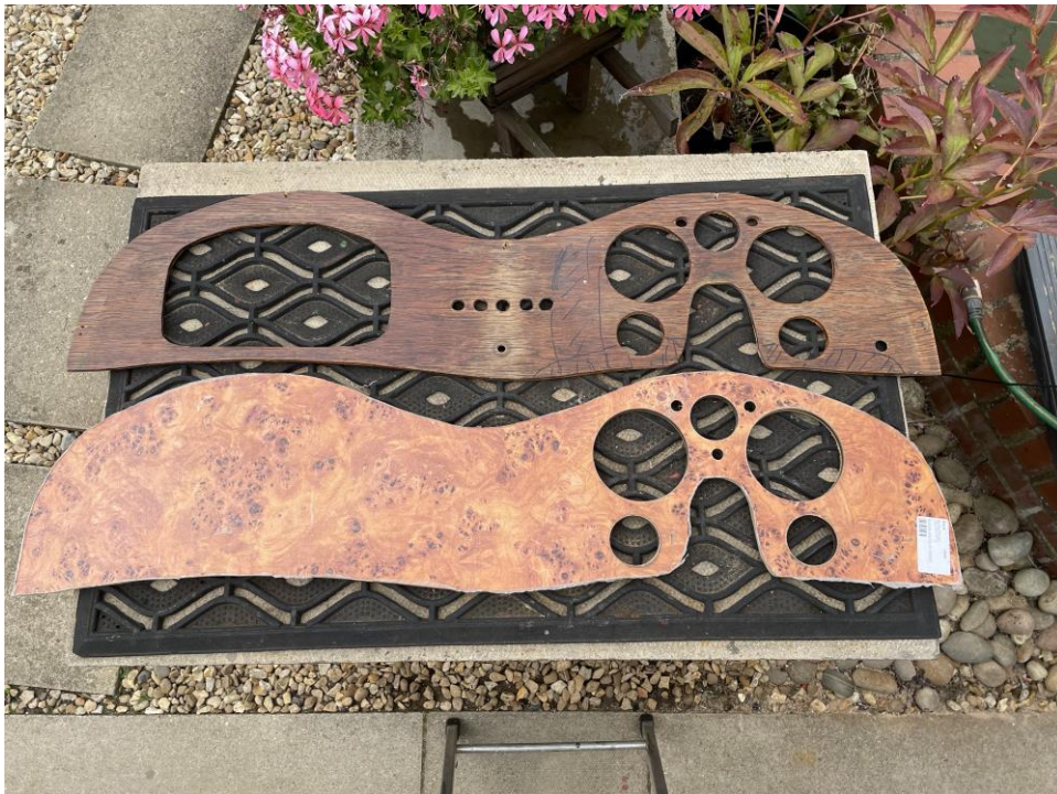
With the gauge and warning light holes cut out.
